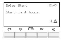
4. Press the OK key. The display shows the DELAY START symbol  $\bigcirc$  and the time until the end of the programme (including period by which the start has been delayed).
